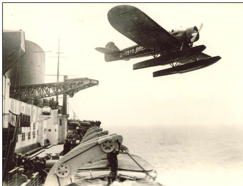
Original photograph of the catapult launching station of the S/S BREMEN. The seaplane was launched when the ship was about 300 nautical miles from its port of call and landed about 2½ hours later in the harbour of New York or Southampton, shortening the travel time of the post bags by two days. Catapulting the seaplane was only performed in calm clear weather.
